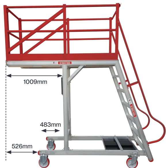
Clearance for Cantilever Platforms
