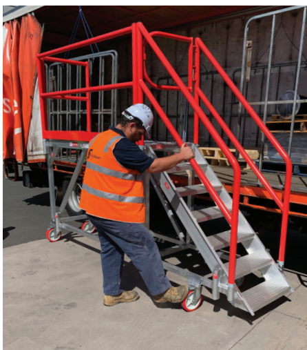
Place in position & lock casters
