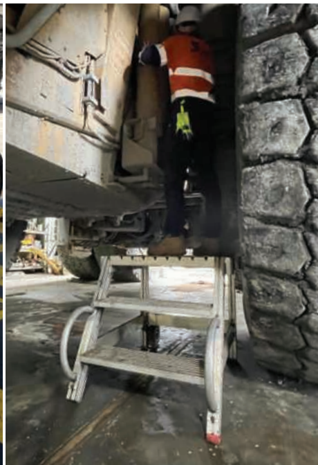
Handles for manoeuvrability, simply lift to engage the front wheels.
