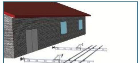
QUICK INSTALL TIP: IF 2 PEOPLE ARE AVAILABLE THEN THE HORIZONTAL RAILS CAN BE FITTED TO THE POSTS WHILE ON THE GROUND. LIFT THE COMPLETE ASSEMBLY INTO PLACE AND TIGHTEN SCREW JACKS UNDER THE EAVES.
