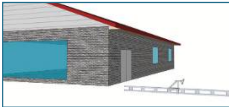
STEP 1 MEASURE THE HEIGHT TO THE UNDERSIDE OF EAVES AND PLACE THE CANTILEVER BRACKET AT CORRECT HEIGHT ON THE EASYRAIL POST.
