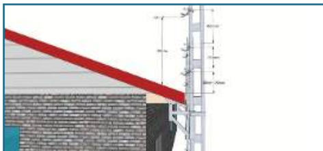
STEP 4 USING A LADDER, PLACE RAIL COUPLER AT A POINT 200mm ABOVE THE ROOF LINE. FIX 2 MORE COUPLERS AT 500mm AND 1000mm ABOVE THIS SAME POINT. ENSURE THE COUPLER "TONGUES" ARE POSITIONED FACING UPWARDS TO HOLD HANDRAIL.
